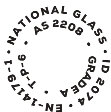
Heat Soaked toughened glass corner stamp verification
