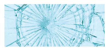
**Heat strengthened glass** is about twice as strong as annealed float glass and is used generally as a protection against thermal breakage. It is not a Grade A Safety Glass.
